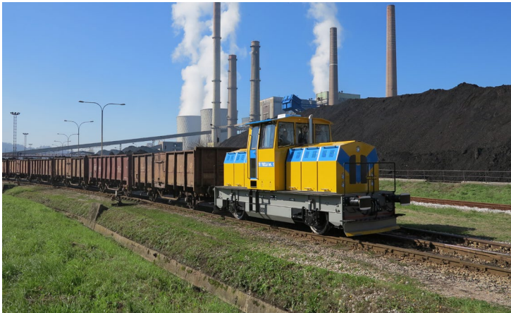
MDD3 is a small 2-axle shunter with great starting tractive effort and variety of speed modifications.
