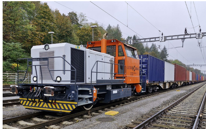
MDD4 is a 42-tons 2-axle shunter homologized for CH, IT, BG. It is designed for heavy shunting service .
