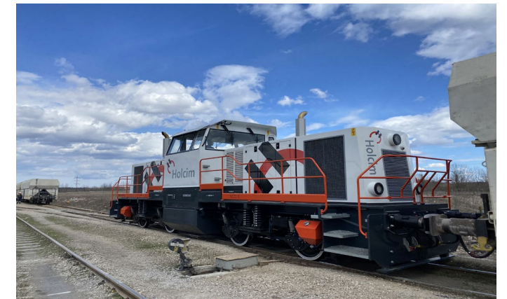
MDD5 is a 4-axle shunter with the best tractive curve in its segment for heavy industrial and light train service .
